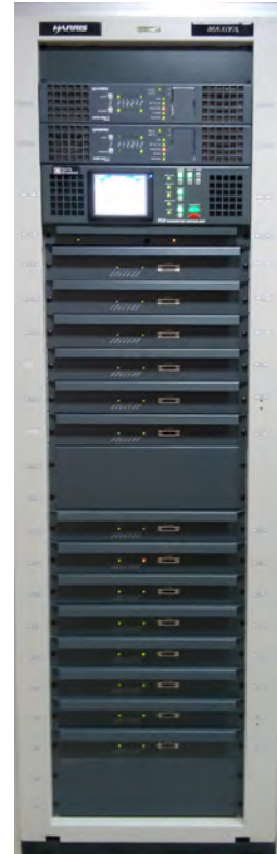
6kW DVB-T2 Transmitter
