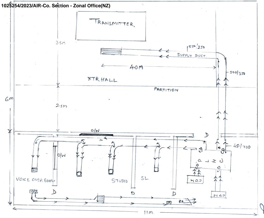
EXTENDED LAYOUT OF SUPPLY DUCT IN XTRHALL & LAYOUT OF SUPPLY RETURN DUCT FOR VOICE OVER BOOTH, STERED TRANSMEMISM
